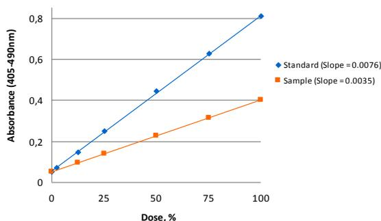
2. Compare the slopes of the standard curve and the sample. In this example the slope of the standard curve is 0.0076 and 0.0035 for the sample curve, resulting in a slope ratio of 0.46 (0.0035/0.0076).
